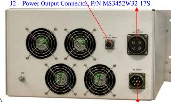
J3 – Control Connector, P/N D38999-20WB35SN
